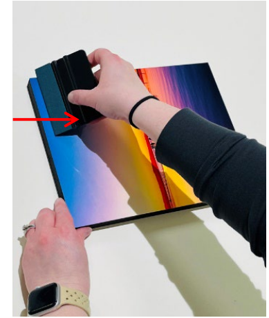
5. Using the soft edge of the enclosed application tool, start at the tacked edge and apply medium pressure across the surface. Use multiple overlapping passes in the same direction.
